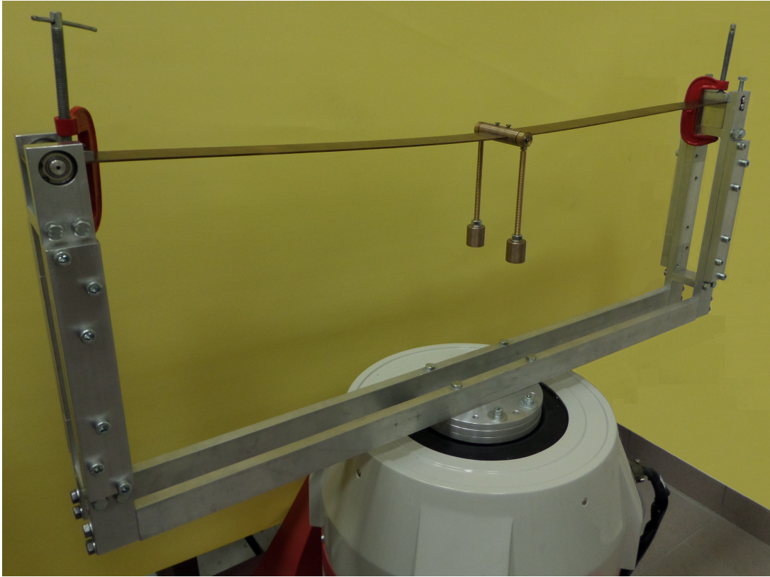
Figure 5.3: Experimental rig consisting of one oscillator node ( n = 1 ).
